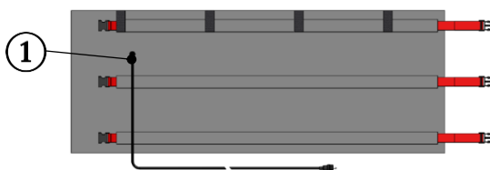
Illustration 1.2: Drum Heater WODH0200-ZP (Exterior) with cable outlet
