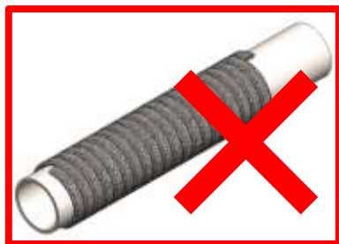
Windings too tight
